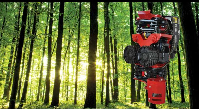
The **SATCO**\* 214 is a small processor with heavy duty features designed to carry out a range of operations from thinning to medium/final cut.
