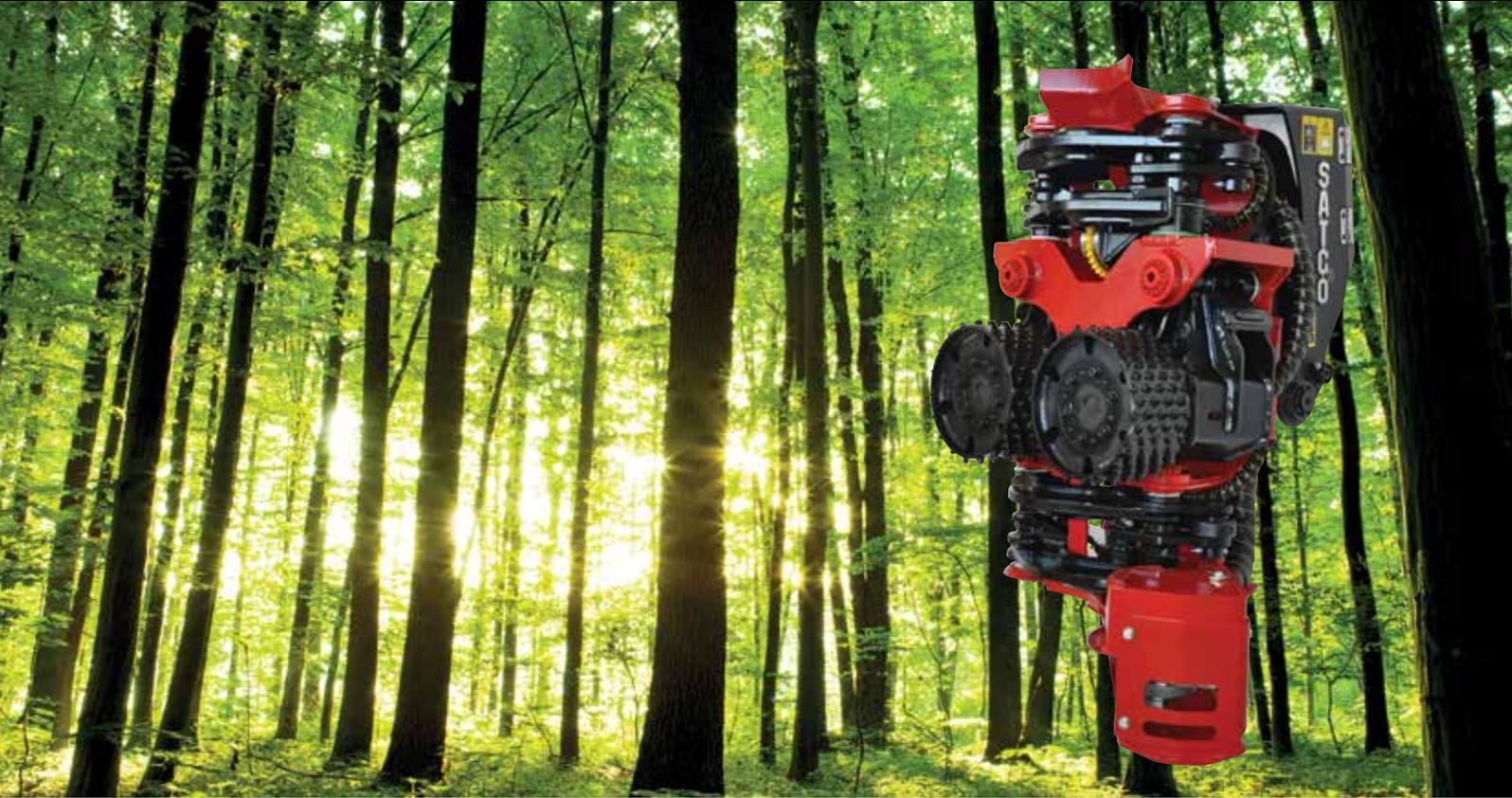
The **SATCO<sup>®</sup>** 214 is a small processor with heavy duty features designed to carry out a range of operations from thinning to medium/final cut.
