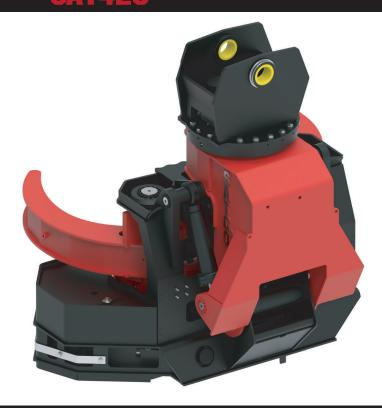
Weighing in at 1548kgs (3412lbs) and requiring 200lpm (52.8gpm)(US) at 280bar (4000psi) this felling grapple can be attached to any carrier in the range of 16-24 tonne. Because the SATCO 420 can be run on a small carrier the horsepower requirement is minimal compared to running a fixed disc saw head. These factors all amount to less carriers stress and great fuel efficiency, giving you the ability to increase your production while bringing down your running costs.
